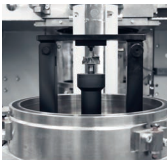
Since the shaft and the turbine wheel are made of different materials, welding these two components together represents a special challenge. MAHLE engineers found the solution: electron beam welding – a process that permits extremely precise and reliable joining.
